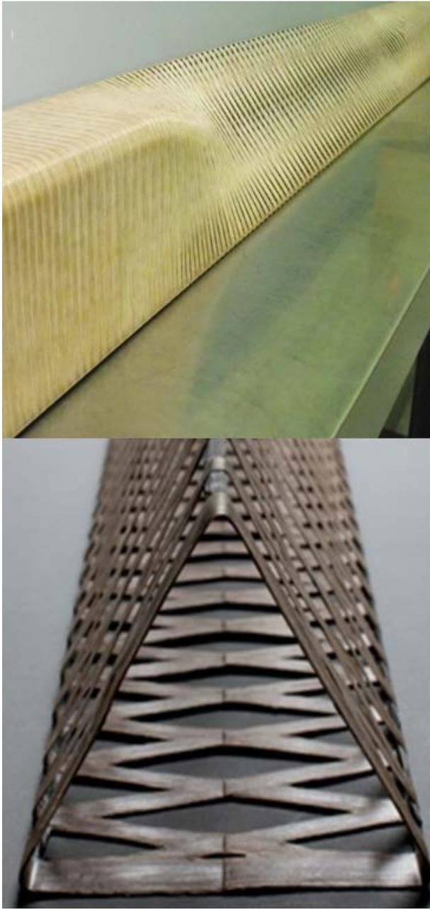
Figure 4. Fiberglass composite beams for a ceiling support concept.
