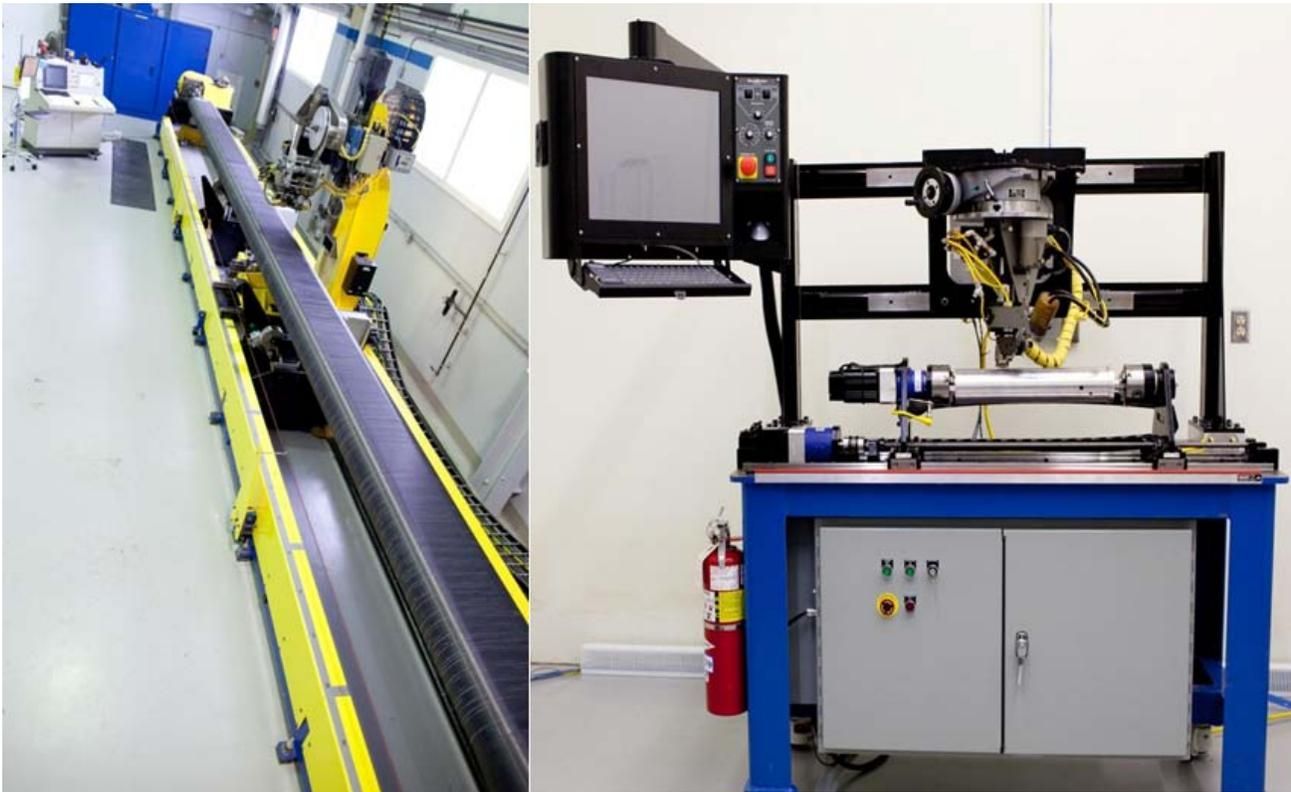
Figure 5. Automated Dynamics' production (left) and lab-scale (right) fiber placement equipment.
