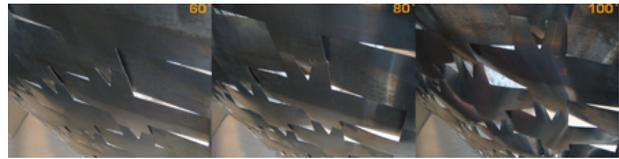
Figure 5. The bimetal tiles in the Armoured Corset started to curl at 80° F.
