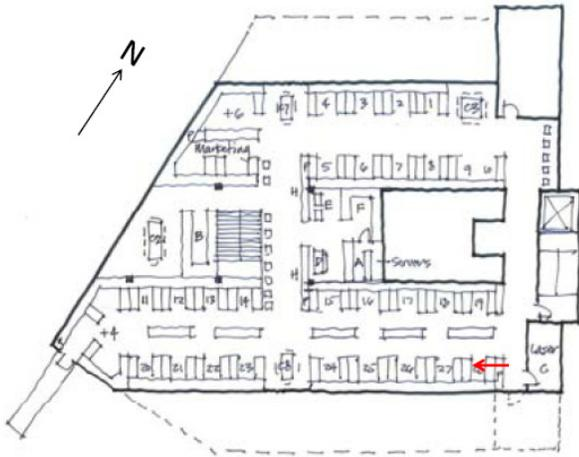
Figure 4. Fourth floor plan of Bullitt Center with workstation location for visual comfort analysis. Diagram: The Miller Hull Partnership.
