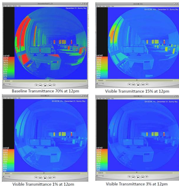
Figure 6. Stills from dynamic luminance maps indicating luminance values in  $\text{cd}/\text{m}^2$  and contrast ratios on September 21 at noon. Note solar disc in glazing at left.
