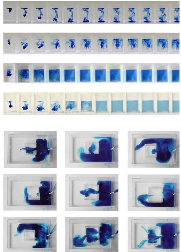
Figure 5. Emilie Tennant and Carin Nakanishi tested the impact of physical obstruction on flow. These tests share a lineage with both Victor Olgay's wind/smoke studies as well as physical models chronicled in *On the Water: Palisade Bay* (see endnote 15). The physical model allows for simple empirical tests for understanding fluid behaviors.
