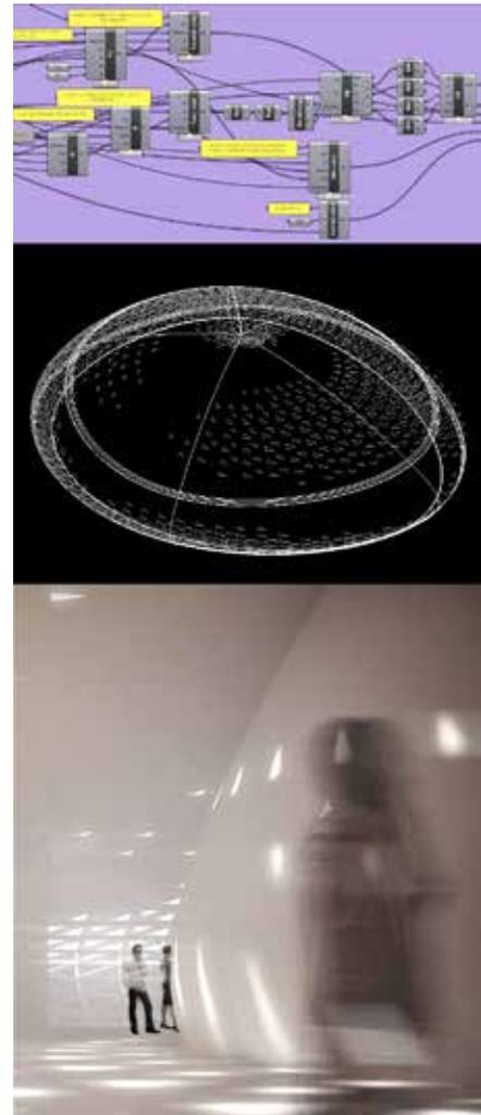
Figure 4: Project 3 using a parametric approach focused around Grasshopper and Galapagos to work with an evolutionary approach. All analyses are generated and assessed within Grasshopper, Images courtesy of Chenqi Jia.
