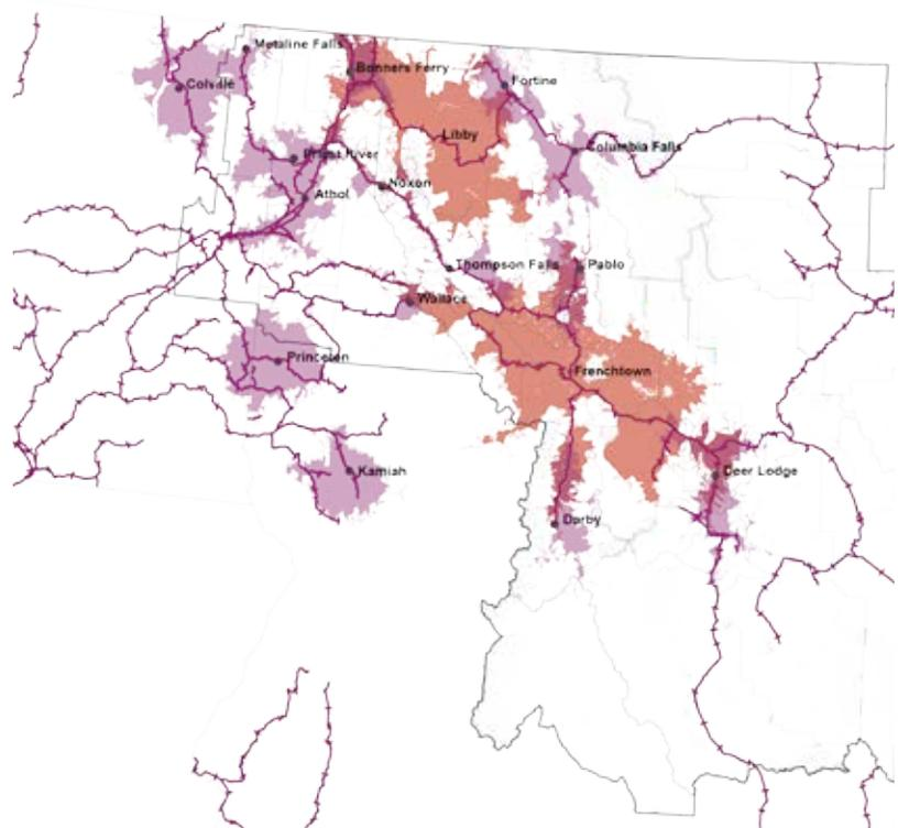
Figure 3: Western Montana Corridor, network analysis of potential woody biomass extraction for establishing techno-economic and LCA parameters. Purple areas indicate 1-hour direct haul to primary processing sites (mills), orange represents 2-hour direct haul to urban secondary processing sites with potential CLT manufacturing capacity (Northwest Advanced Renewables Alliance, 2013, analysis credits Jon Potter, WSU).
