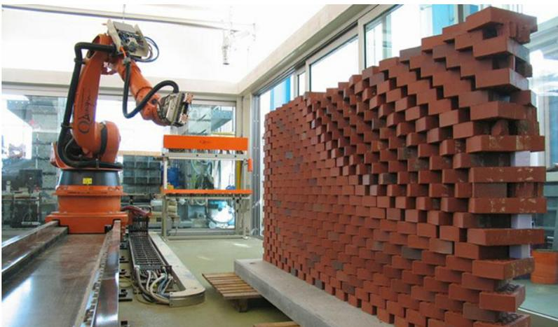
Figure 3: Programmed Wall, 5-axis robot building
