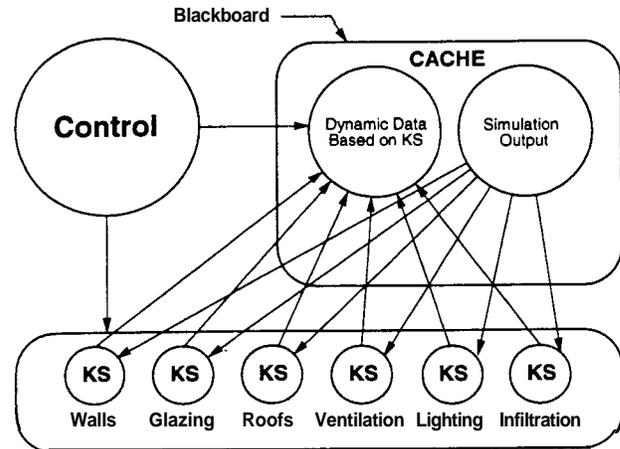
Fig. 4. The Components of the IBEDO System.
