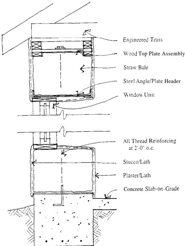
Fig. 3. Typical Wall Section
