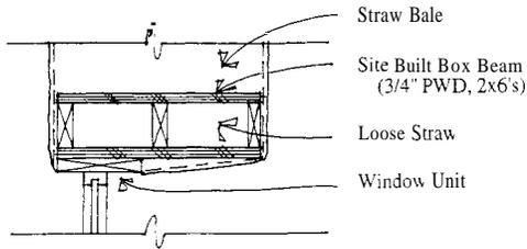
Fig. 4. Alternate Box Header Detail
