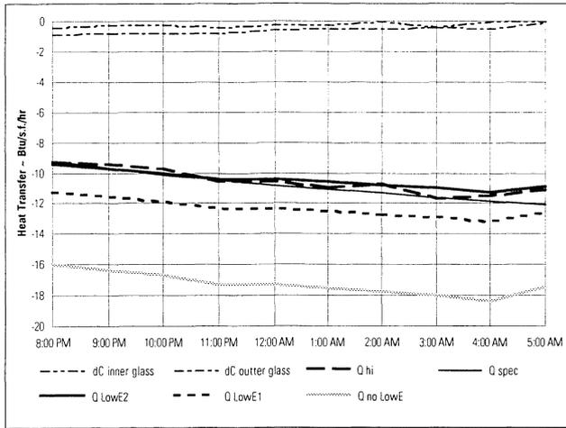
Figure 6: Heat flow across the glazing estimated from measured surface and air temperatures.
