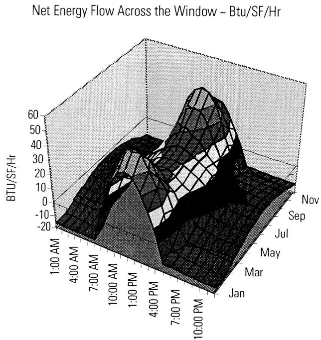
Figure 8: Average hourly heat flow across glazing for the year, an output graph from *Glazing.xlsx*.
