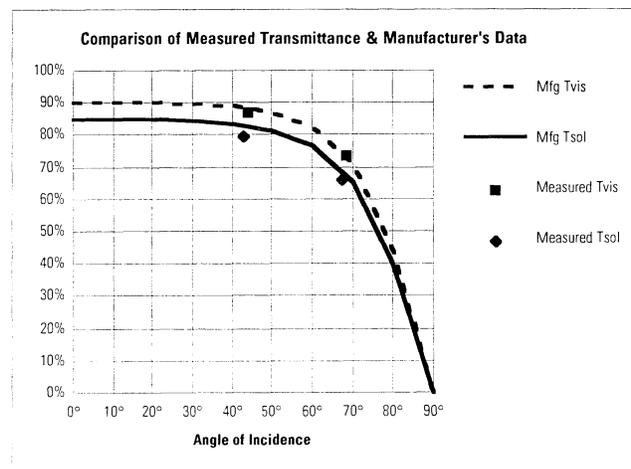
Fig. 5. Comparison of manufacturer's data and field measurements. The angle of incidence of solar radiation is accounted.
