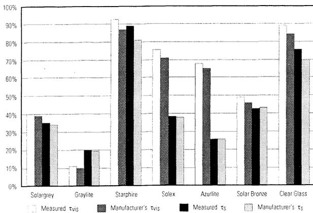
Fig. 2. Comparison of measured transmittance (visible and solar) with manufacturer's data for a variety of glass types. The manufacturer's data was drawn from the **WINDOW 4.1** database.
