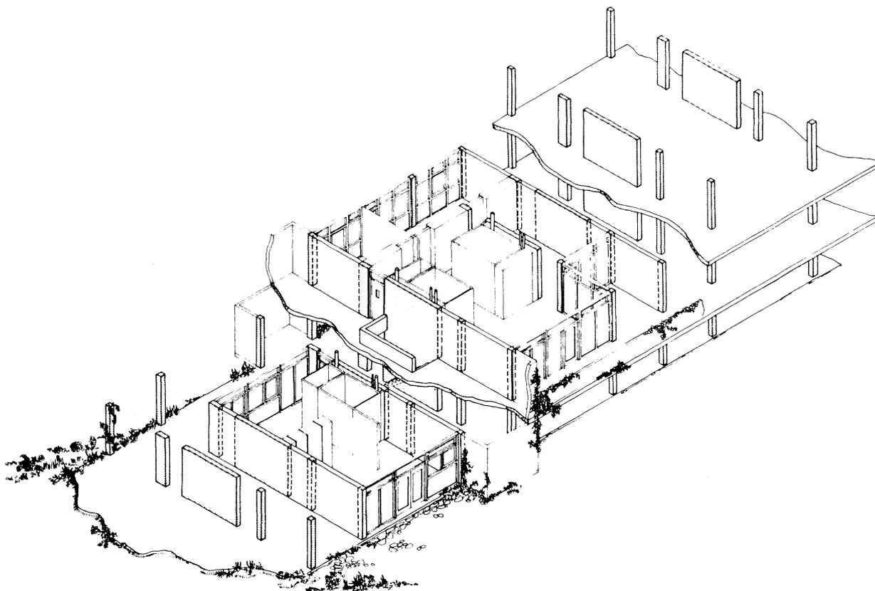
Fig. 3. Bijlmer support system, City of Amsterdam, 1970, illustrating Habraken's theory of supports.<sup>23</sup>
