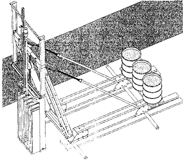
Fig. 2. Isometric view of lifting and drilling rig. Drawing- Caitlin Moore.
