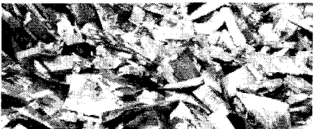
Fig. 8 Low-grade waste paper from food boxes was used in initial IAA building material grant research.
