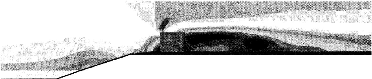
*Fig. 1. Simulated hurricane force wind flow over a low rectangular building located downwind of an escarpment*
