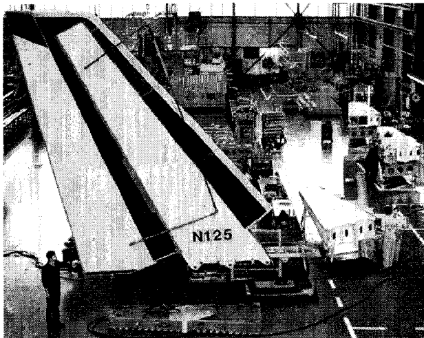
25. Wing of an Airbus A320/200, load-bearing structure made out of composite fabric material. Daimler-Benz Aerospace.
