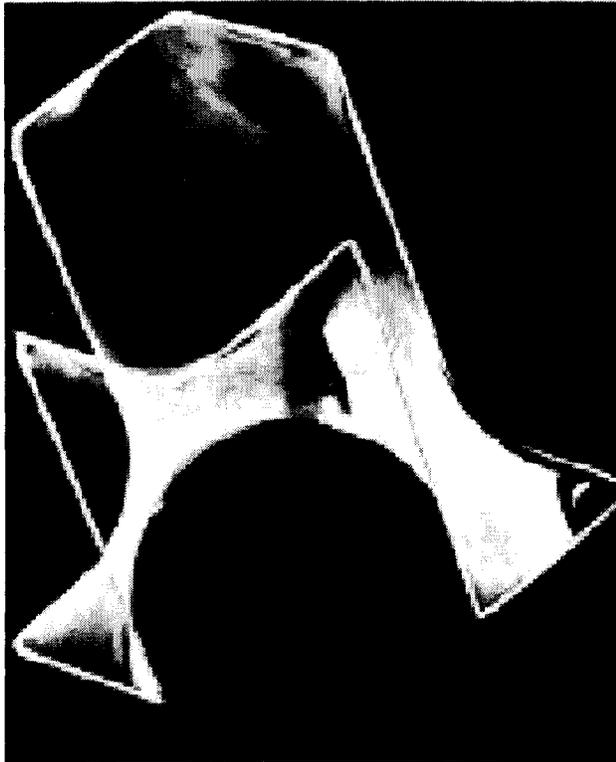
Figure 3. Experimentation with soap bubble membranes.
