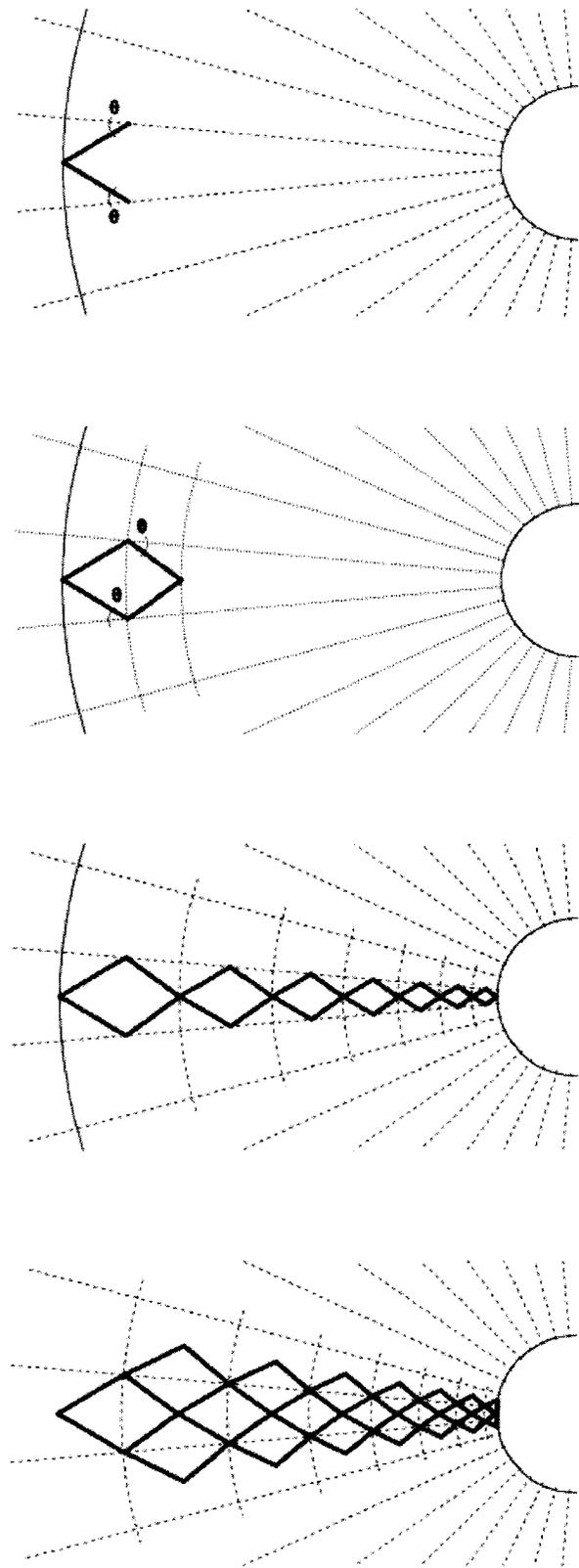
Fig. 3. Proportioning system used by Nervi on the lamella dome projects.
