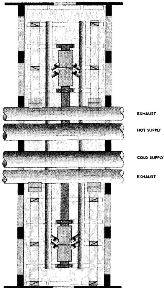
Fig. 5. Typical bay of interstitial space showing modular air handling scheme as developed by Fred Dubin. Major trunking runs through the center of each bay, with mixing boxes located toward the access corridors. Alternating supply and exhaust registers allowed rooms as small as ten feet square to be fully ventilated.
