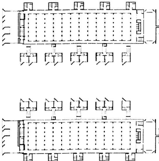
*Fig. 4. Plan of interstitial level showing (left to right) office blocks, major interstitial 'rooms', and mechanical wings. Each block is flanked by studies and service towers.*
