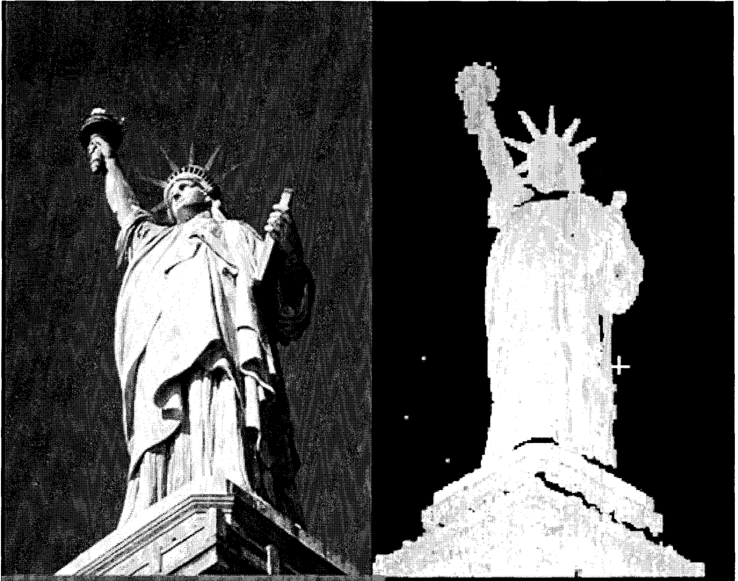
Fig. 8. Model showing surface mapping and areas of missing data.
