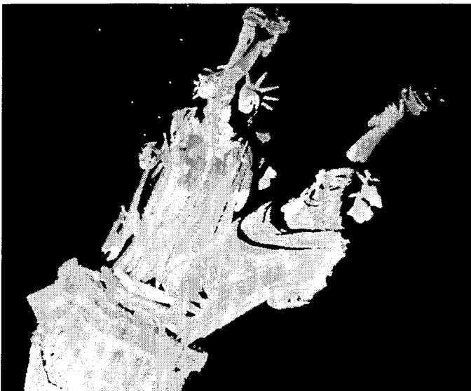
Fig. 5. First attempt to register four scans together shows errant target registration.
