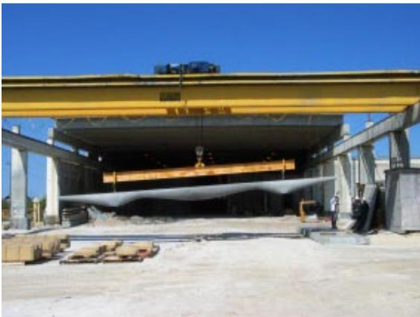
*Figure 1. First 12 metre (40 ft.) prototype reinforced concrete beam cast from a prestressed fabric form at the Conforce Structures factory, Winnipeg, Manitoba, 2003.*
