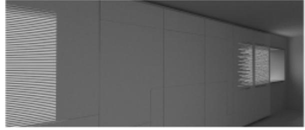
Figure 11. Engraved MDF panels with integral light screens
