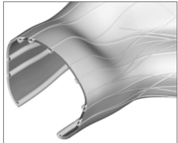
The XURRET System experience shows how a final ornamental effect emerges from a programmable design environment, which combines mimetic intentions with the abstraction of mathematical rules, in a continuum between conception and manufacturing. The final built components are monolithic and made from a single material –concrete- that blends structure and surface, volume and texture, form and ornament (Fig. 6).
