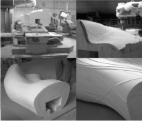
Figure 6. The final XURRET System components are monolithic and made of concrete, blending structure and surface, volume and texture, form and ornament.
