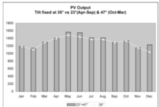
degrees on September 21st. The increase is mainly due to improved efficiency in May, June (23 degrees tilt angle) and December (47 degrees tilt angle), see Figure 12.
