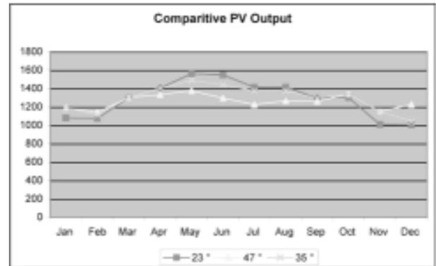
Figure 12: Monthly values of annual predicted electric output from the PV array with panels fixed at a 35 degrees tilt angle (line) and panels at 23 degree tilt during the summer half and 47 degrees tilt during the winter half of the year (bars).
