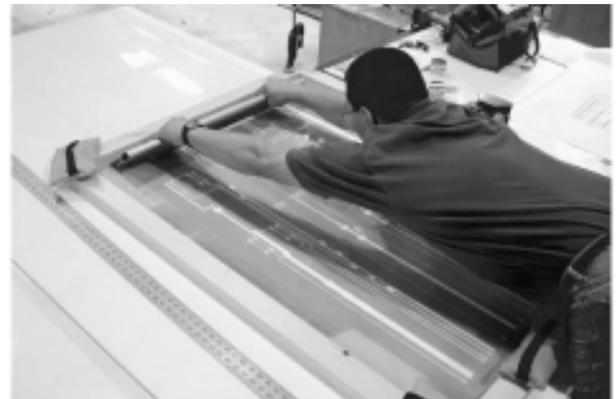
*Laminating the components. Image by ILC Dover, Inc.*
