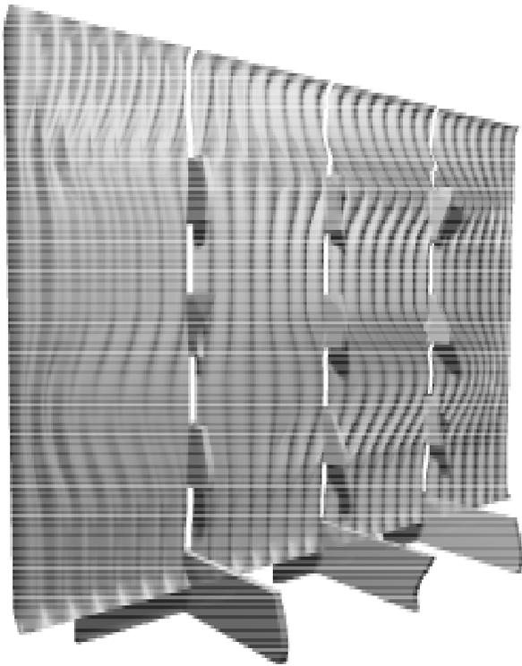
prove that by producing the formwork from designer-produced architectural models, the difficulty of drawing interpretation and time consumption of formwork building by contractors would be significantly reduced if not eliminated. The resultant reduction of labor and precision of formwork would make CNC driven concrete work financially comparable to and formally more flexible than traditional concrete work.
