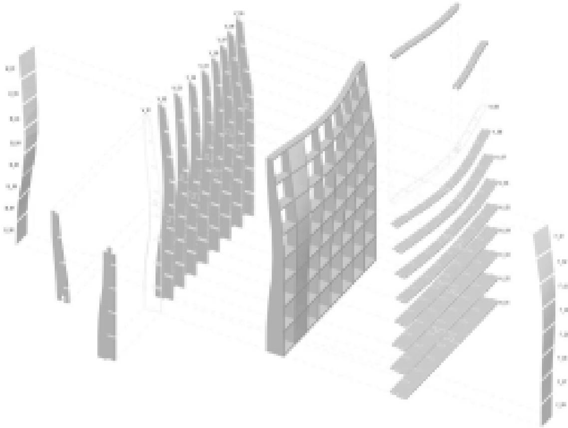
physically moved. Medium Density Fiberboard, for financial reasons, was substituted for aluminum components and much of the steel bracketing as well as the concrete slab, which was substituted with 12 sections of milled 3/4" MDF.
