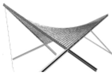
The dynamic nature of the form was further accentuated by placing the raking columns on sloping concrete buttresses in the ground, reminiscent of arch bridge construction, clearly articulating the force line from the structure to the foundations. The out of balance forces resulting from imposed snow and wind loads are understood from the need to provide a 3<sup>rd</sup> vertical support located at the rear of the stage.
