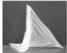
The model in Fig 8, began to describe what the chosen solution became, a model formed out of paper, that describes an overall hyperbolic form, as a consequence of origami folding technique. Curiously Fig 8, aptly exemplifies the principle described earlier, whereby macrostructure (shell) is derived from microstructure (skin).
