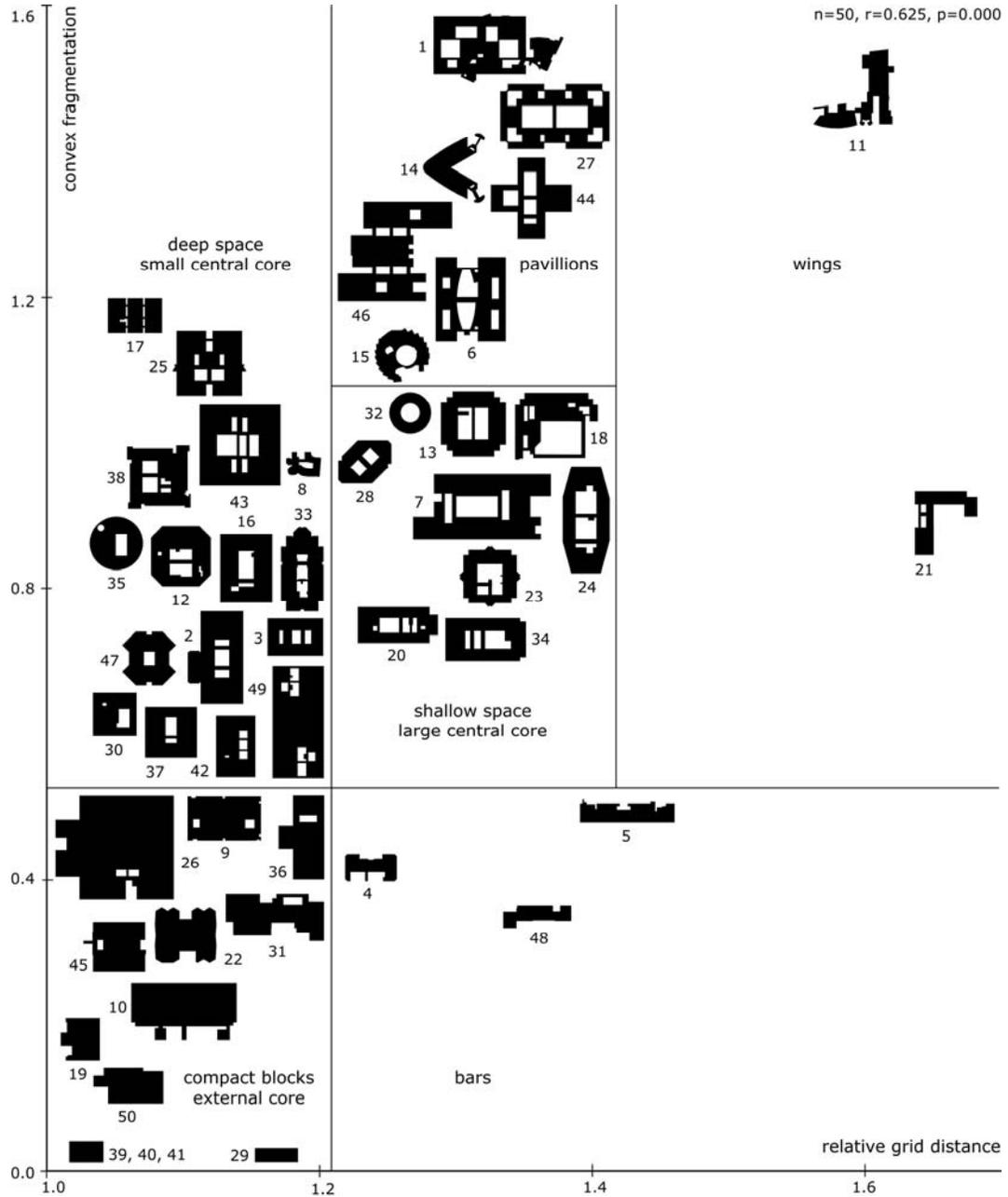
Figure 1. Fifty floorplate shapes compared according to compactness and fragmentation
