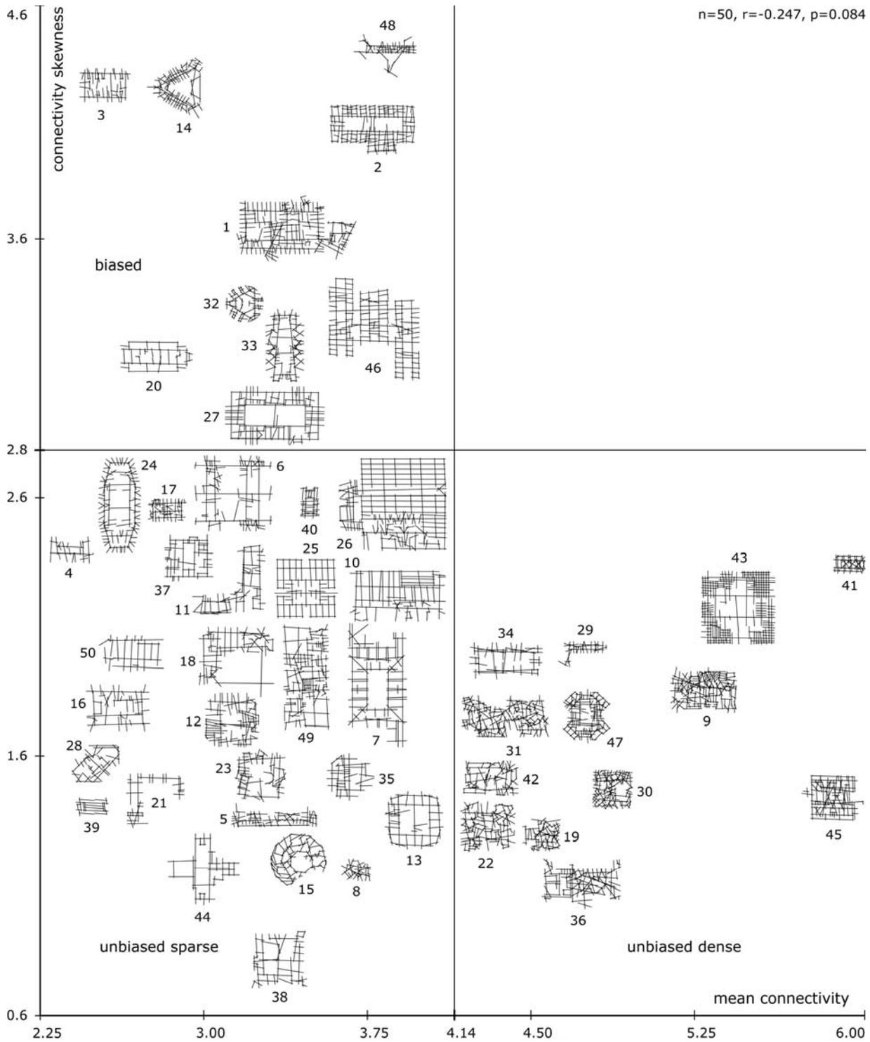
Figure 2. Fifty office layouts compared according to connectivity and connectivity bias
