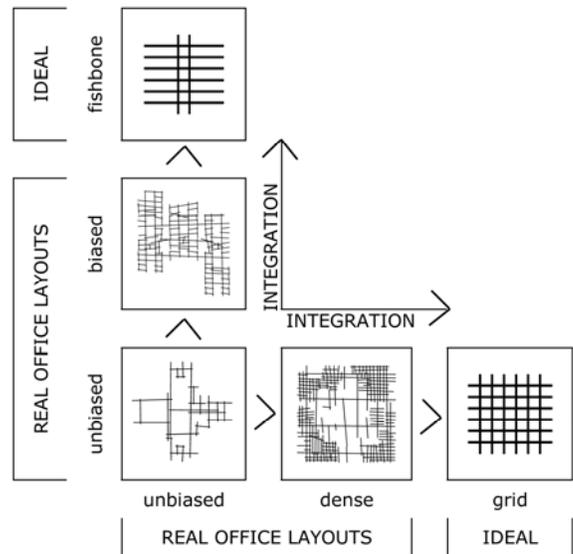
Figure 3. Two ideal layouts representing two selected types of real layouts and two alternative ways of increasing integration
