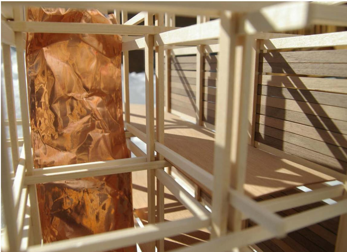
Figure 3 : Copper as a vertical reflector of light in a wooden physical model.
