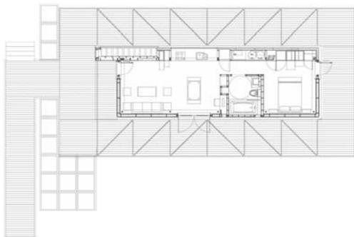
Fig. 4. In the plan one can find efficient space planning, a very compact and multifunctional north "core" wall, a bathroom "core" separating public and private, west, south and east insulated translucent wall assemblies, the wrap-around deck with converted truss framing, and the landscape water filtration planters.
