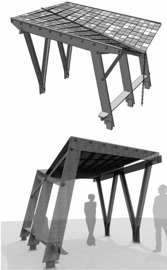
Fig. 3. First proposal (below) refined to add roof overhang and rain-chain (above).
