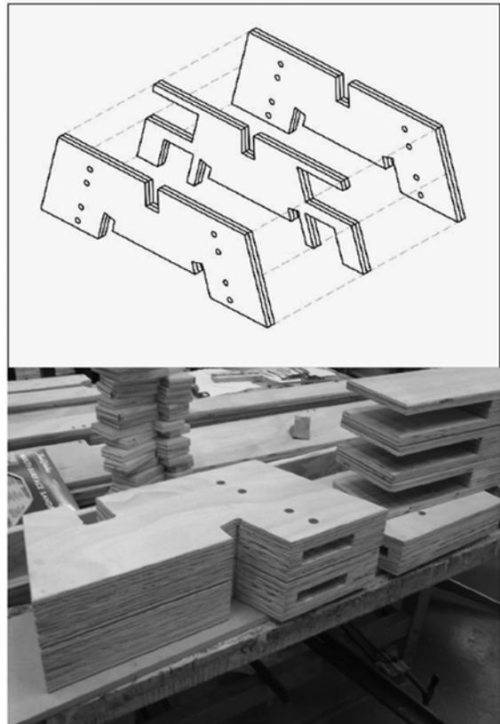
Fig. 4. Complex laminated plywood blocks.
