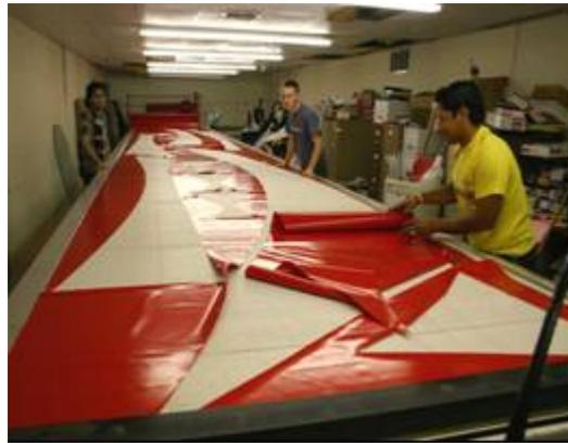
Figure 2: Membrane Cut to Pattern.
