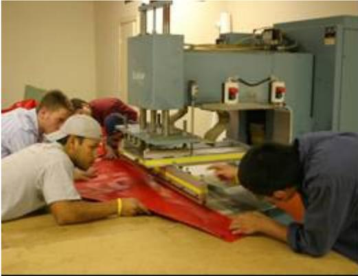
Figure 3: Radio Frequency Welding of Membrane Panels.
