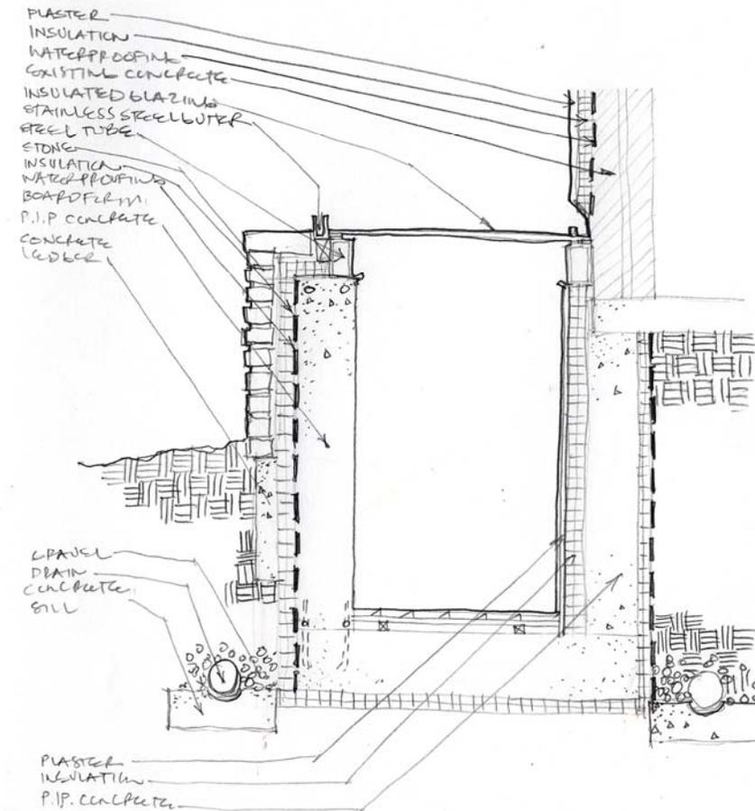
Fig. 5. Student's in-class sketch of a poured-in-place concrete passage at the lower level of the concrete case study, a house outside Zurich, Switzerland
