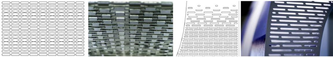
is maintained within the digital model. Changes in the design can be made and their effects on the components are manifest with different toolpaths to be sent to the CNC fabricators to cut the patterns.
