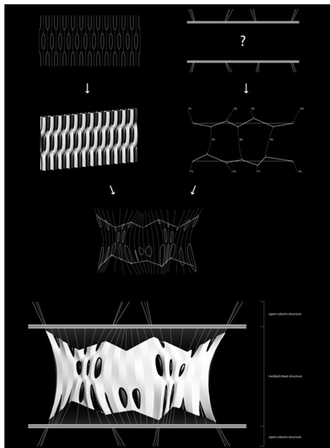
Figure 2. A graphic pattern (left) and moment diagram (right) are combined in a thermoformed wall prototype.
