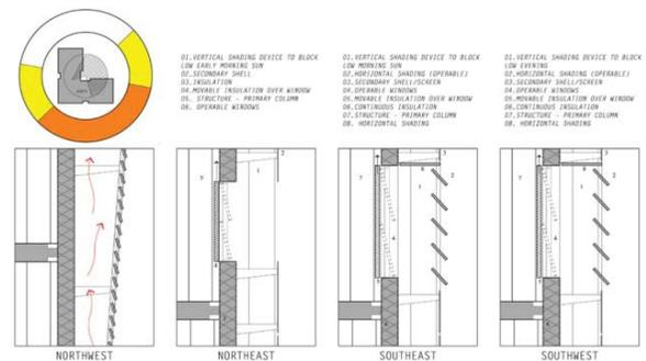
Fig. 2. Schematic envelope assemblies
