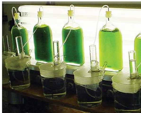
Figure 3 "DIY Algae/Hydrogen Bioreactor", (Franceschini, 2004) [NATURE, VOL 414.15, NOVEMBER, 2001 www.nature.com]
