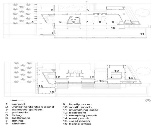
**Figure 2:** Plans of the house (ground floor above, second floor below)
