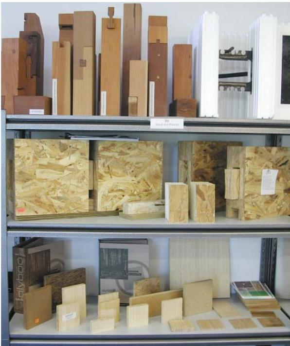
Fig. 1. Samples in the library show the various compositions of wood products.
