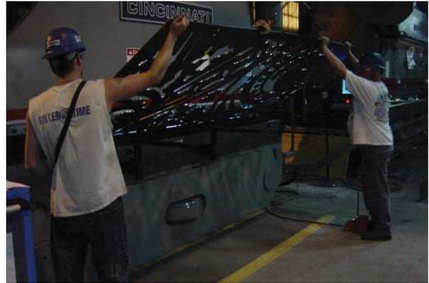
ton NC press brake for accurate bend angles. Panel sizes also needed to respect the brake opening and accessibility issues. As the brake is predominantly used with steel these issues translated back to the design models and simulated with the laser cut chipboard model panels.
