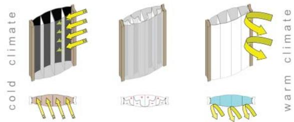
Figure 4 - Thermally responsive low-pressure pneumatic skin, invented by Nikolaus Laing
