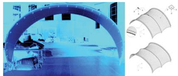
Figure 3 - Lightweight Structures Unit research: Fabric web braced arch (L), Studies of double curvature morphologies (R)
