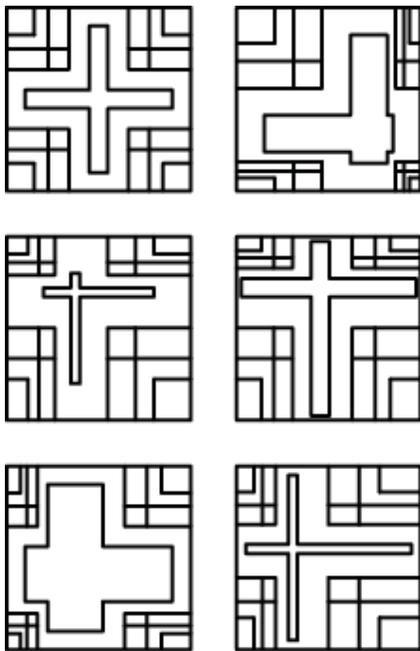
Figure 3: Original Frank Lloyd Wright design of the Millard House textile block and new designs from parametric variations.
