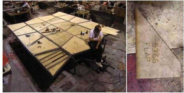
Figure 2 - Fabrication of the Mobile Stage (L) and CNC cut Jig for laying out and welding the trapezoidal frames (R)
