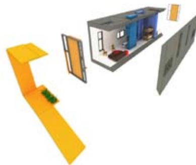
**Figure 5** Unit components
