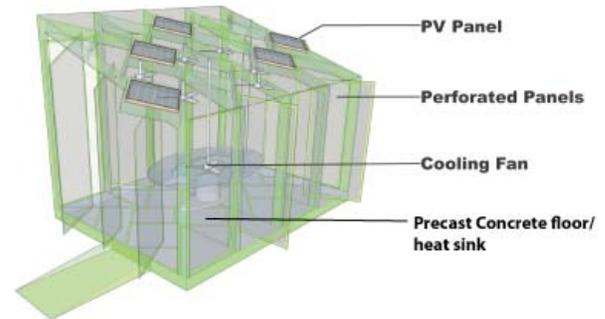
Figure 2. Early design stage design 45-degree PV panel assimilation.
