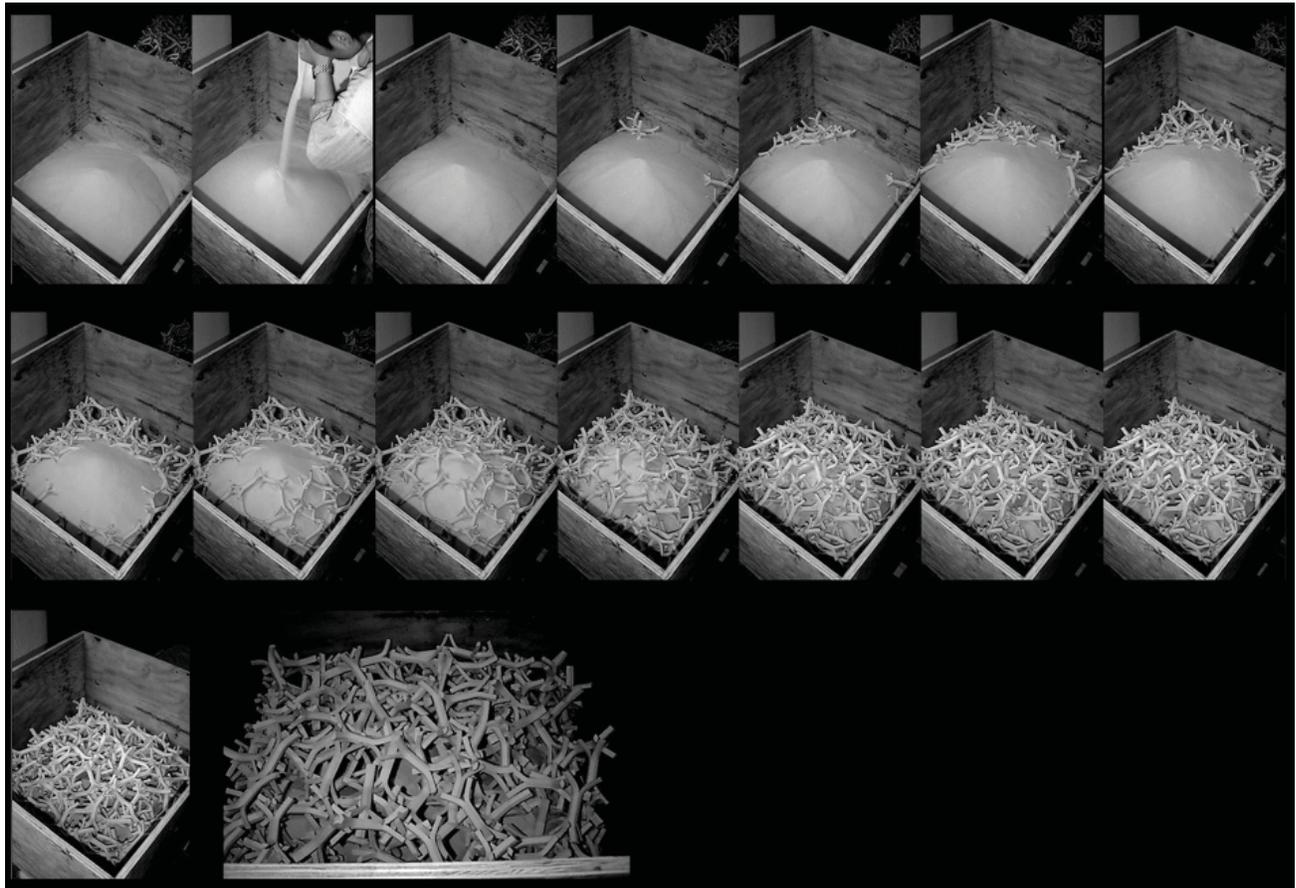
Figure 3. Tumbling Units, Construction Sequence via Silica-sand Formwork
