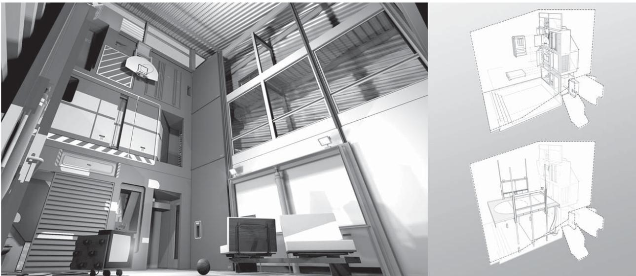
Figure 3. The entire floor plate of this single-person residence is a hydraulic elevator platform. As the occupant moves the floor up and down alongside a vertical program wall it becomes functionally re-programmed, which dramatically alters the character of the space and also serves as a continuous index of daily activities. (Doug Jackson)
