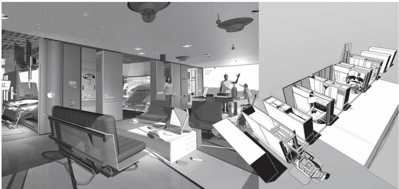
Figure 5. This project features a system of program cabinets that can be slid back and forth within the available volume. The occupants are able to create program-specific spaces between the cabinets as desired, and to eliminate that space and rededicate it to another program as interests change simply by repositioning the cabinets. (Jones, Partners: Architecture)
