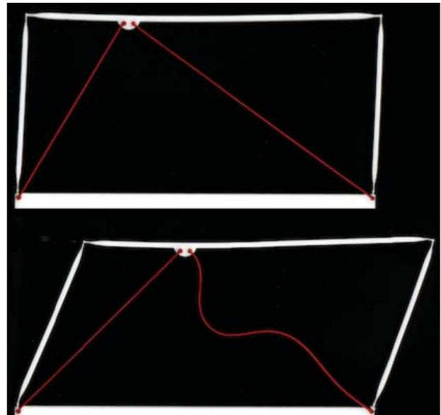
Figure 1. Portal Frame in Unloaded and Loaded Condition
