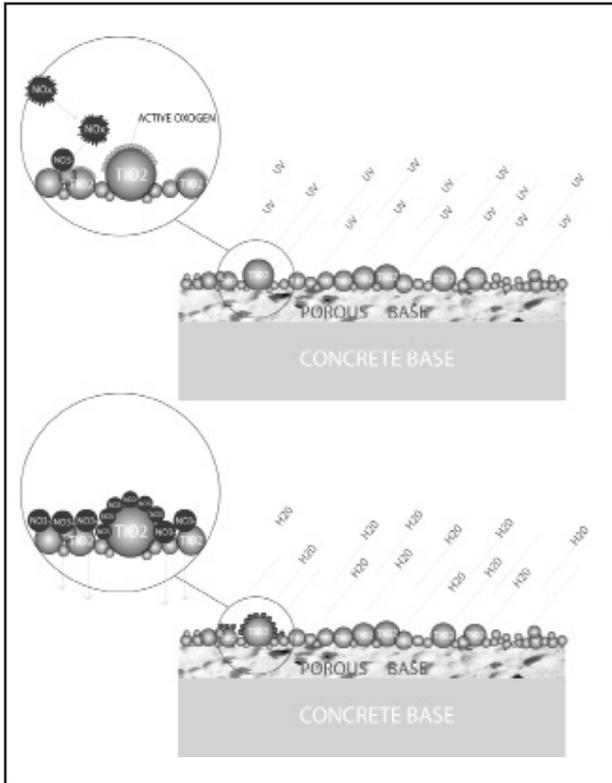
Figure 1: TiO<sub>2</sub> and Concrete Photocatalytic Reaction, source: (Author 2009)
