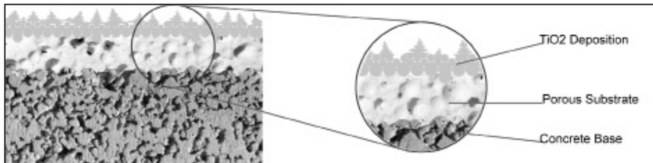
Figure 2: Composite lamination illustrating micro-topography source: (Author 2009)
