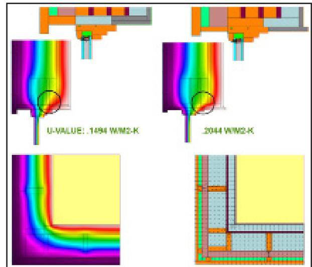
Figure 5: Thermal bridge studies with Therm 5.2 by studio students showing various envelope conditions. Window header (top), typical framing at stud with diffusion-open wood particle panel adjacent to rainscreen cavity (bottom).
