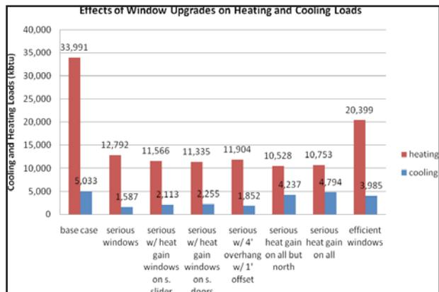
Figure 5 - Effects of Window Type on Total Heating and Cooling Loads. (Source: HEED/Excel)
