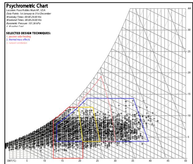
Figure 2 – Psychrometric chart showing passive heating strategies. Passive solar heating is outlined in red thermal mass in blue and natural ventilation in pink. The comfort zone is outlined in yellow. (Source: Weather Tool)
