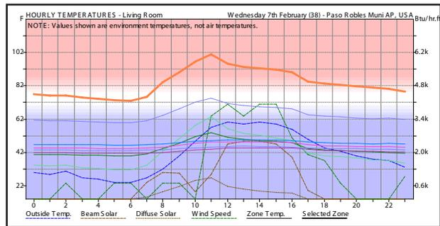
Figure 4 - Estimated Hourly Temperatures on the peak coldest day, with living room shown in orange (Source: Ecotect)
