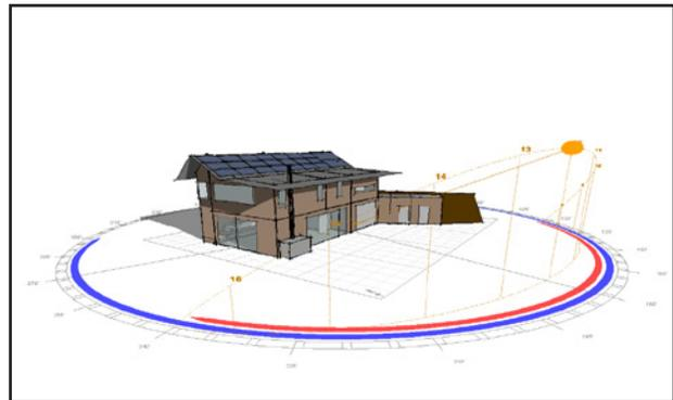
Figure 3 - Model showing sun shadows on December 21 @ 12:00PM (Source: Ecotect)
